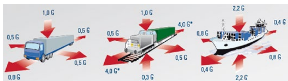
Fig. 5 : Accelerations in accordance with means of transport
