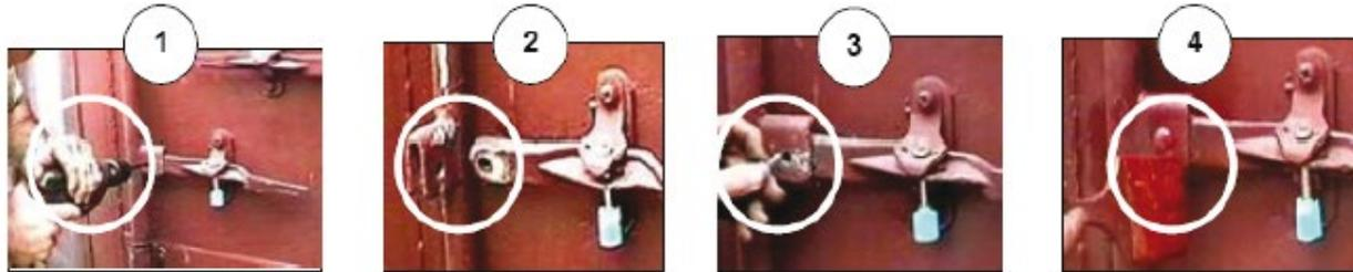
In relation to the bolt-type seal: position the top of the cap pointing upwards. This will make it more difficult for plunderers, who fill it with a liquid (acid or liquid nitrogen) so that they can open and close the seal invisibly.
